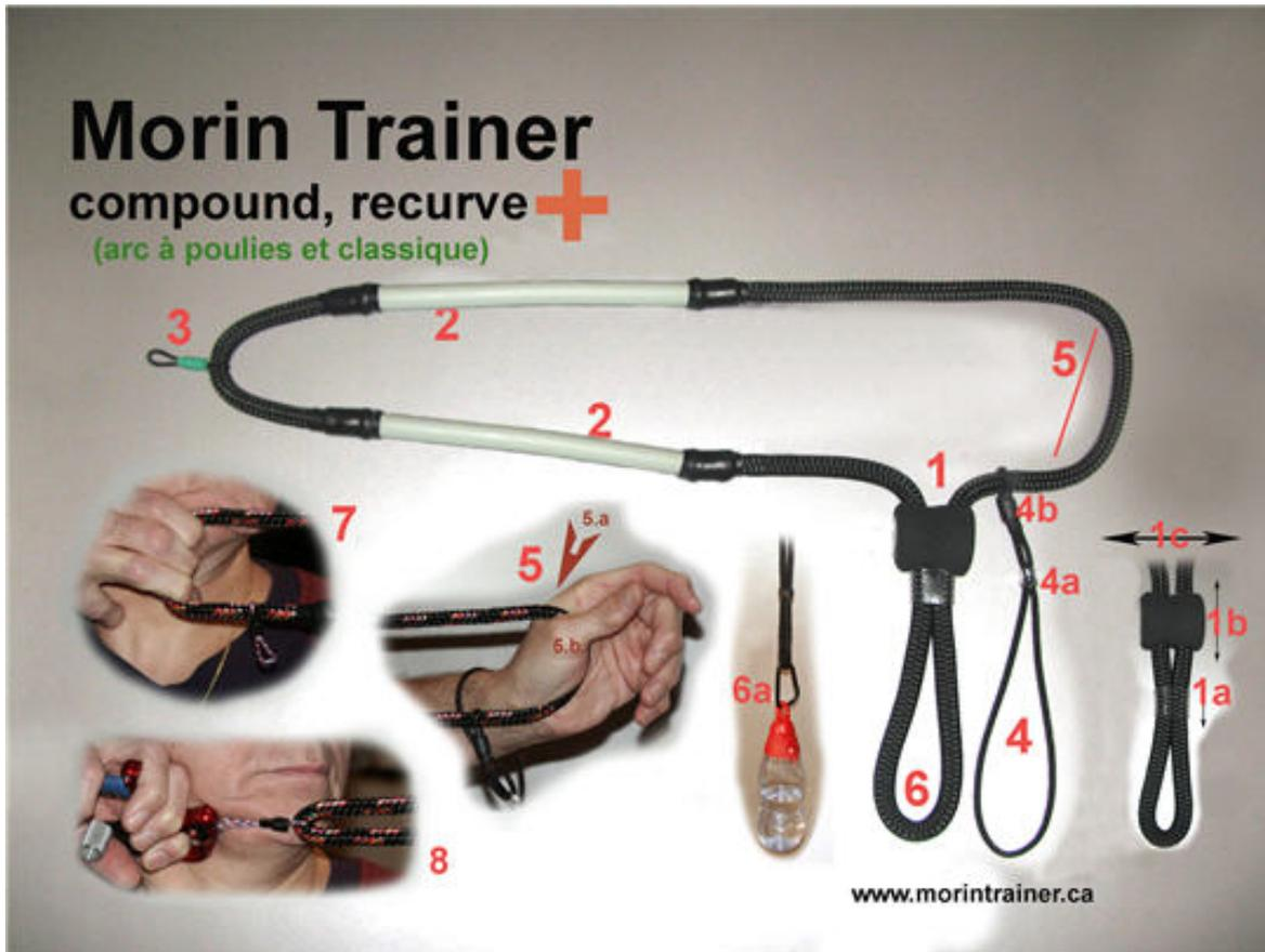
1- The adjustment node makes it possible to modify your draw length. The photo (cut away view) shows the operation for the draw length adjustment. To adjust your draw length, you only have to pull on the 1.a part to unlock and then you pull down the 1.b part to lengthen or to go up to shorten it. Moving part 1 near the bow hand will limit the projection of this piece.
